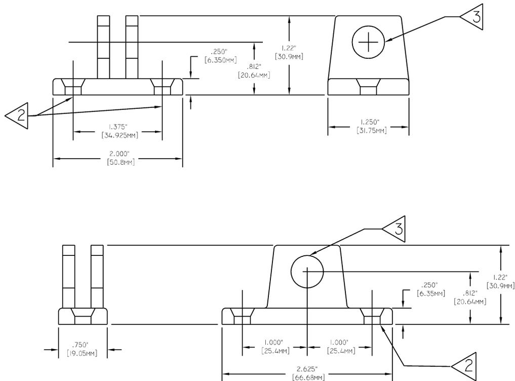
LONGITUDINAL Latch Block-Eye Bolt shown at top.
