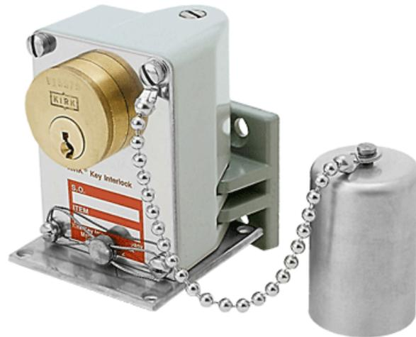
The Type DY2 interlock is made for loose fitting access opening doors. It has two parts: a main body and a latch block-bolt eye. A stainless steel mounting plate is attached to the base of the main body as pictured.
